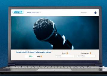
Unique to Wavin, the SoundCheck Tool simulates system acoustics in a final installation and calculates noise levels based on individual parameters. In just six clearly defined and intuitive steps, you can get the answers you need to see if your design meets regulations.
